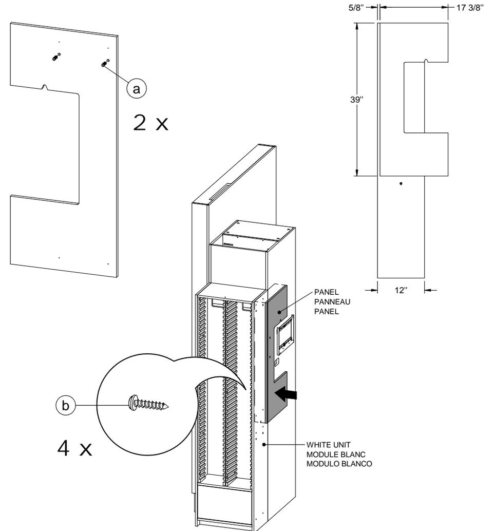
Procedure for installing the display
