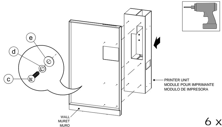
Procedure for installing the display
