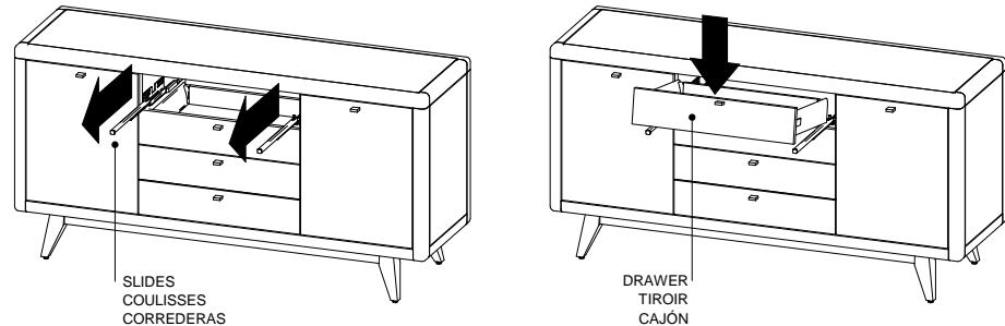
· Hold front of slide under drawer and pull until the mechanism is engaged. Verify that the grey clamp under the drawer is correctly engaged into the slide (see the picture). Repeat for the second side of the drawer.
